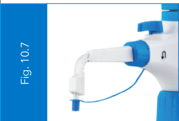
Reattach the cap to the discharge tube. (Fig. 10.7)
