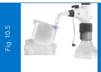
Hold the discharge tube orifice against the inner wall of the appropriate receiving vessel. (Fig. 10.5)
