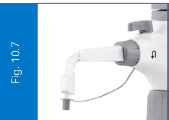
Reattach the cap to the discharge tube. (Fig. 10.7)
