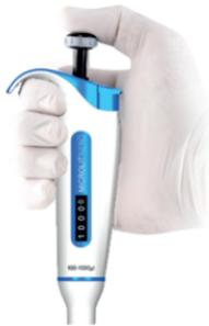
5. Make sure that the tips, the micropipette and the reagent/solution are at the same temperature.
