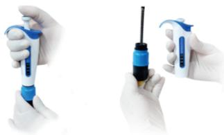
Step 2: Pull the lower ejector housing to separate it from the upper ejector housing.
