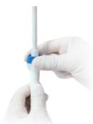
Step 4: Screw the tip ejector assembly in the clockwise direction to the upper housing.
