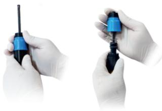
Step 3: Rotate the tip cone in the counter-clockwise direction to separate it from the piston.
