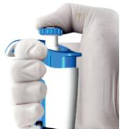
1. To aspirate the liquid in the tip, press the plunger to the first stop and Immerse the pipette tip vertically in the liquid.
