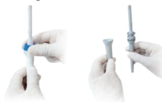
Step 3: Pull out the o-ring seat and turn the tip cone upside down and retrieve the o-ring.
