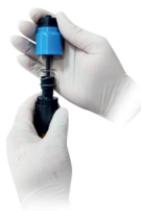
Step 3: Assemble the ejector housing to the upper housing by rotating in the clockwise direction.
