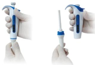
Step 2: Rotate the piston assembly counter-clockwise to separate the piston from the tip ejector housing.
